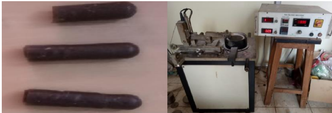
Figure 2: (a) WSP-polyester composite specimens prepared for sliding wear test (b) Pin-on-Disc machine
